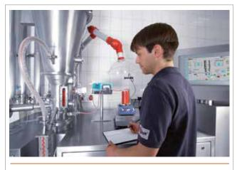
Figure 2. Flexible plant concept for batch and continuous fluid bed and spouted bed processes. (Copyright: Glatt)
