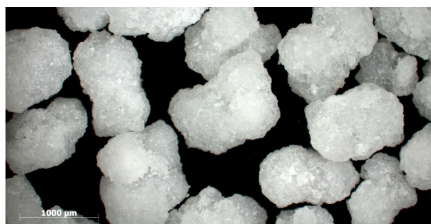
Figure 2. Microscopic picture of granules produced during the feasibility study intended for use in compacted fertilizers.
