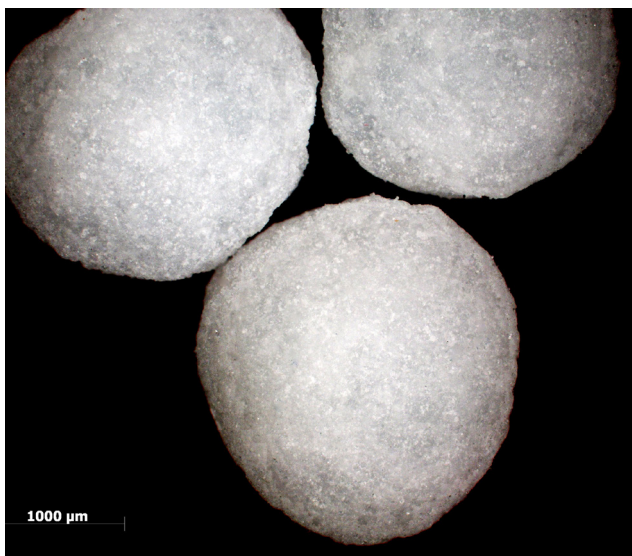
Figure 4. Microscopic picture of granules produced during the second test series intended for use in fertilizer blends.
